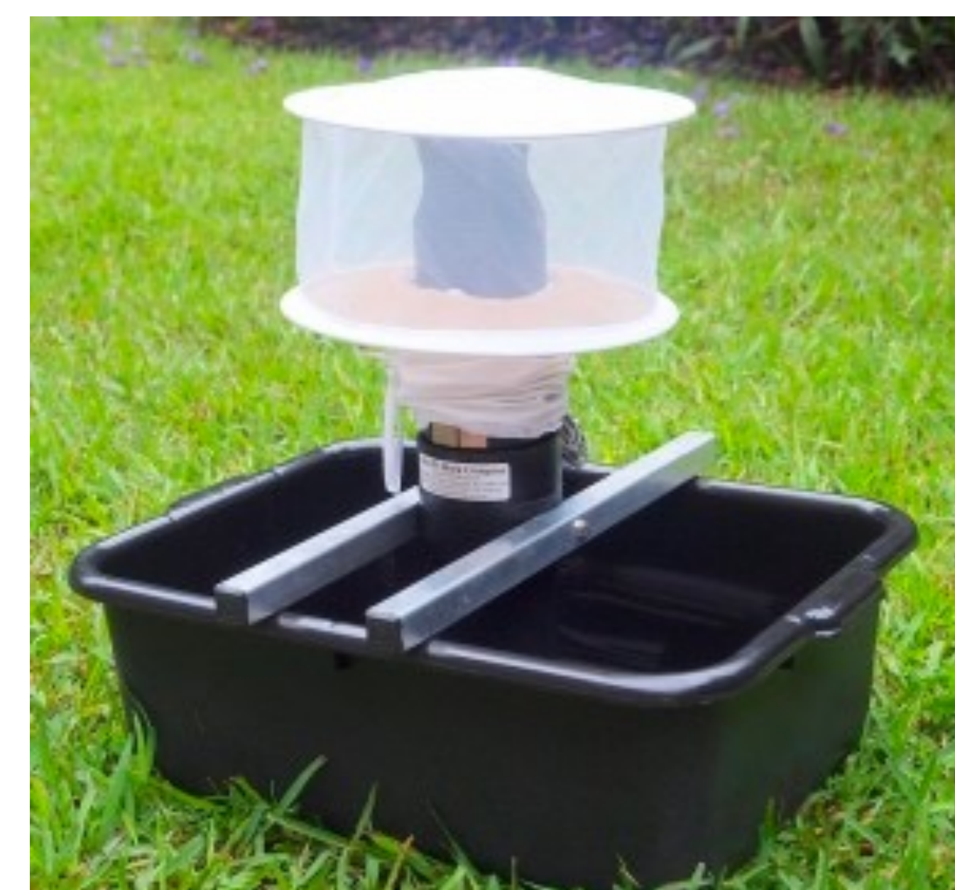
Image of a gravid trap, which is used by NOMRTCB to conduct mosquito surveillance. This trap is specifically designed to catch gravid, or egg carrying, females.
